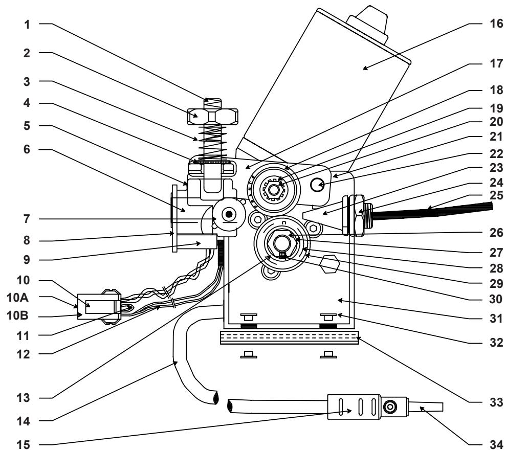
FIGURE C1 - WIRE DRIVE ASSEMBLY (SN-138C24B)
