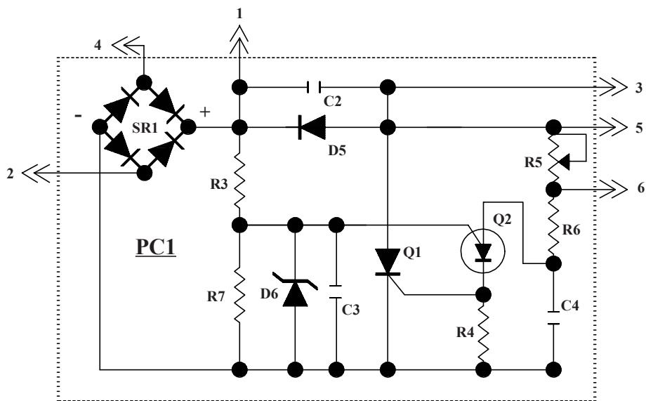
FIGURE 1A - SCHEMATIC, WIRE FEED CIRCUIT BOARD
