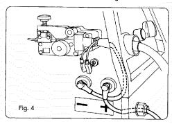
Use only diam. 0.9 flux cored wire that complies with thestandard AWS AS 20 E71 TII or E71 TGS, suitable for use without shielding gas.
