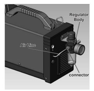
Attach the Air Line to the connector on the side of the Regulator Body. The connector is designed to securely hold the line after inserting. Gently pull on the line to ensure it is firmly held.
