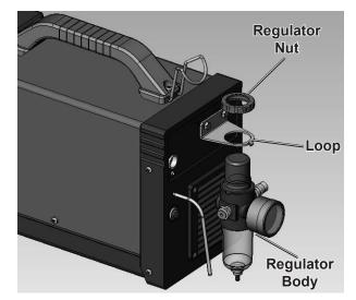
Slide the Regulator Body up through the Loop on the back of the Cutter and attach in place with the Regulator Nut as shown in the illustration above. The Loop is keyed so that the Regulator should only align in one position.
