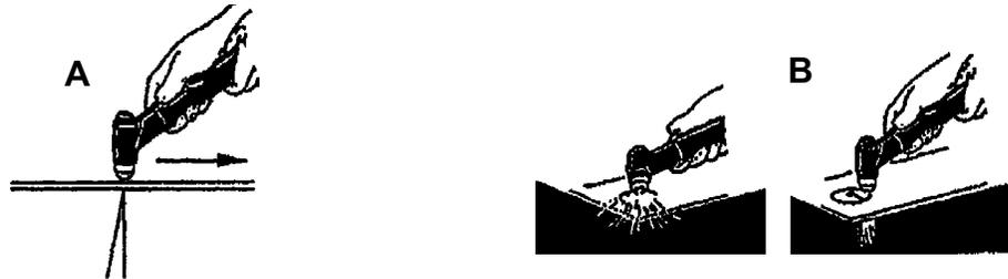
In some cutting operations, it may be necessary to start the cut from a point away from the edge. See illustration "B" above. The backfire from this operation could shorten the life of the torch components, so it is recommended to do this cut as fast as possible.
