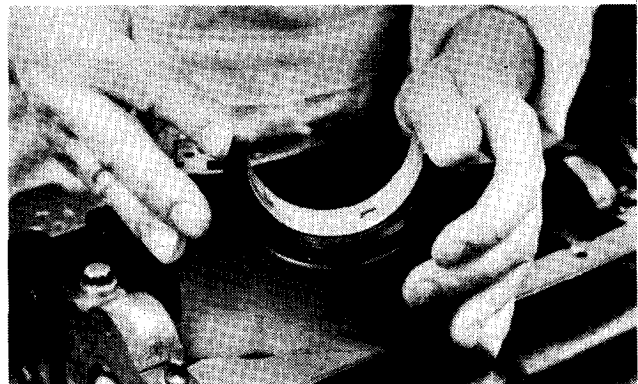
Rear Main Bearing Cap and Filler Block
