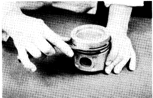
Checking Ring Clearance in Groove
