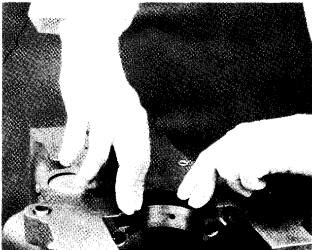
Crankshaft Oil Seal in Block
