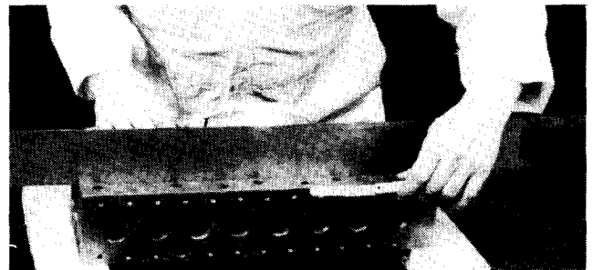
Checking Cylinder Head Flatness Lengthwise
