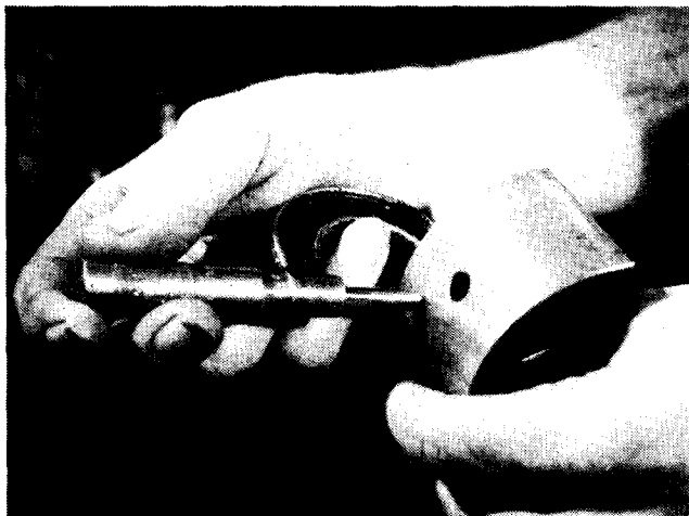
Measuring Bearing Thickness
