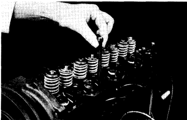
Removing Push Rod from Ball Socket of Tappet
