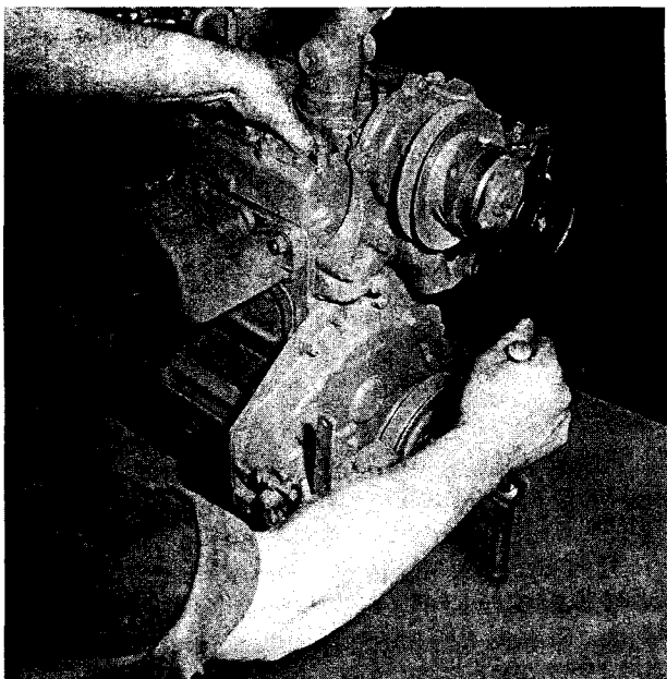
Figure 104 — Checking No. 1 Cylinder on Compression Stroke
